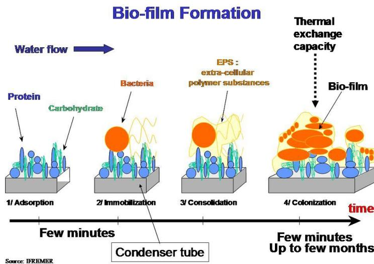
Fig.1. Biofilm formation in a condenser tube. (From Wikimedia Commons).
